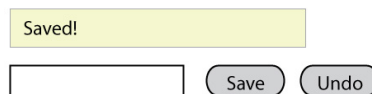
Figure 4.5: After the third step of the form submit process in Figure 4.4, an undo button appear next to the save button. If the user presses the undo button, the posting of the text will be undone.
